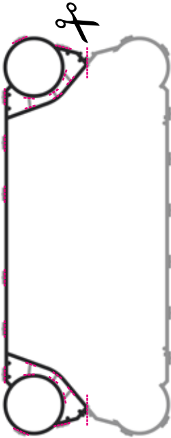
1) Cut two gaskets into half, and cut away the marked tabs.
